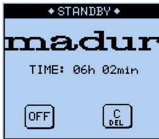
By pressing [**OFF**] the instrument can be switched off completely. If [**C**] is pressed the instrument switches ON again. If the instrument is in **STANDBY** mode for more than 8.5 hours it switches off automatically. It is highly recommended to carry out a [calibration of the oxygen](#) sensor when re-activating the instrument.
