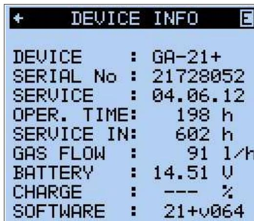
The **DEVICE INFO** screen shows the serial no. of the instrument, the date of the last service, the operating time, the time until the next service, the speed of the sucked flue gas , the battery charge, the battery capacity and whether or not the communication with the **madCom** PC software is locked.
